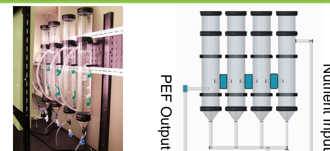
Figure 3. (Right) Constructed airlift, (Left) airlift CAD.
